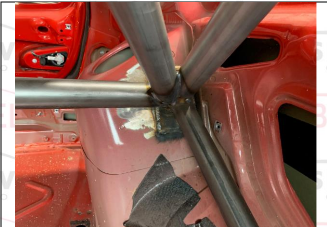
PHOTO 5 REAR BACKSTAY TO BODYSHELL ATTACHMENT
